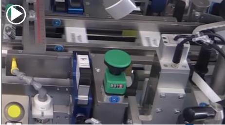
Camera 1 Check of serialized code and data on carton flap (operator side)
