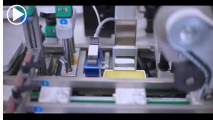
Camera 3 Check of serialized code and data on carton flap (opposite to the operator side)
